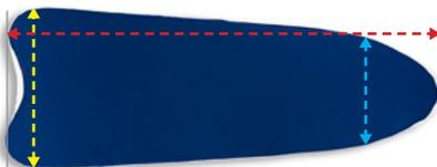
If you cannot find the model number on a laydown press, please provide measurements. Provide length, from tip to tip, and the width at the widest and narrowest ends. See diagram to the left. *Specify if your measurements are for the top or bottom of the machine.*
