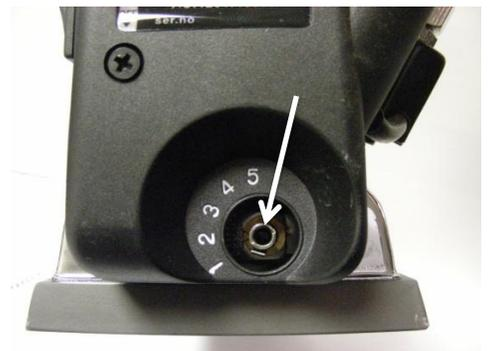
17-Unscrew indicated screws to adjust cover in order to center the stem (if necessary).
