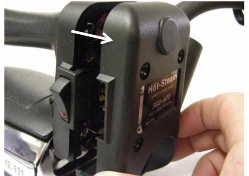
7- Remove 2 wires screws.
