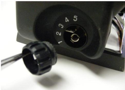
5-Remove *Main Switch Cover* screws (3)
