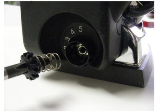
4-Remove the *Temperature Dial Housing*.
